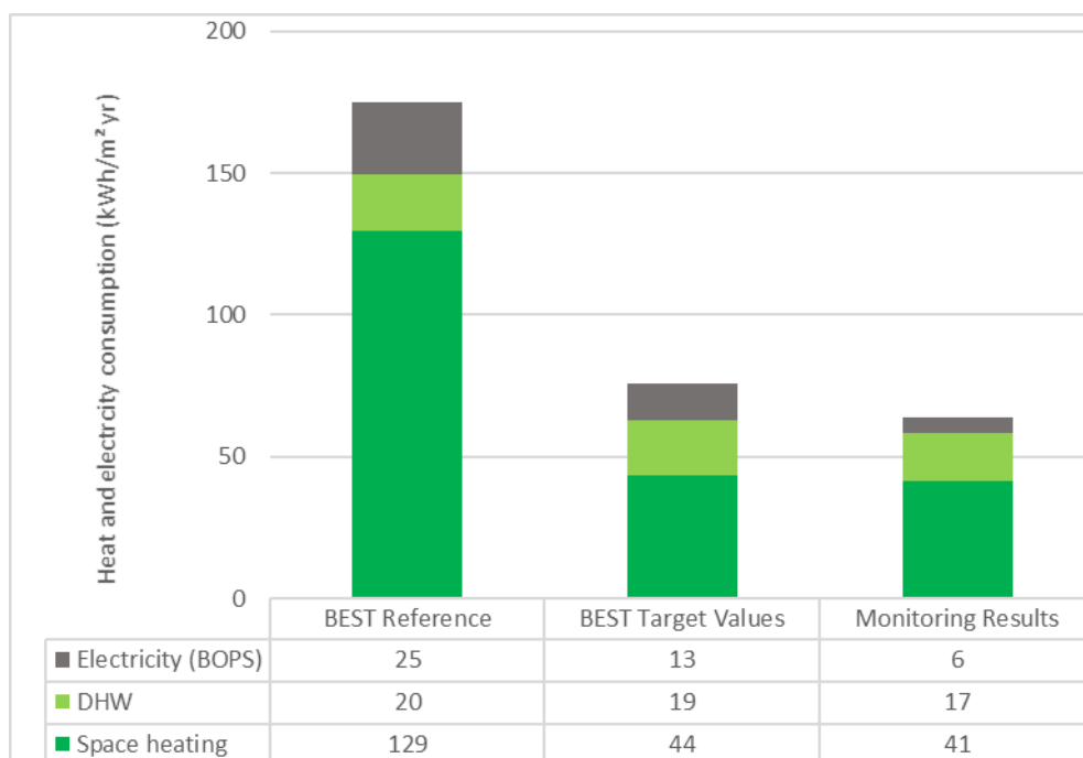
Figure 1: BEST Reference, BEST Target Values and Monitoring Results (2019 resp. 2020) of heat consumption for space heating and DHW and electricity consumption (BOPS) in READY (floor area-weighted average)
