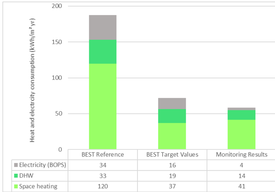
Figure 45: BEST Reference, BEST Target Values and Monitoring Results (2019 resp. 2020) of heat consumption for space heating and DHW and electricity consumption (BOPS) at the RDS in Aarhus (floor area-weighted average)
